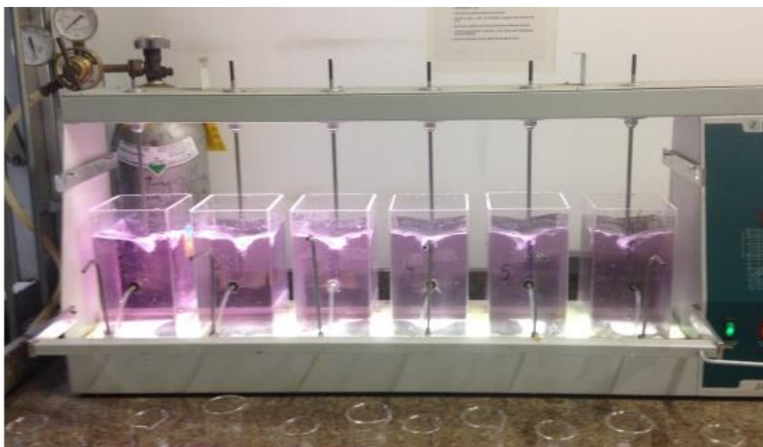
Figure 6: Water in the jar test equipment with six different PAC concentrations and addition of \text{KMnO}_4 = 2 \text{ mg/l} .
