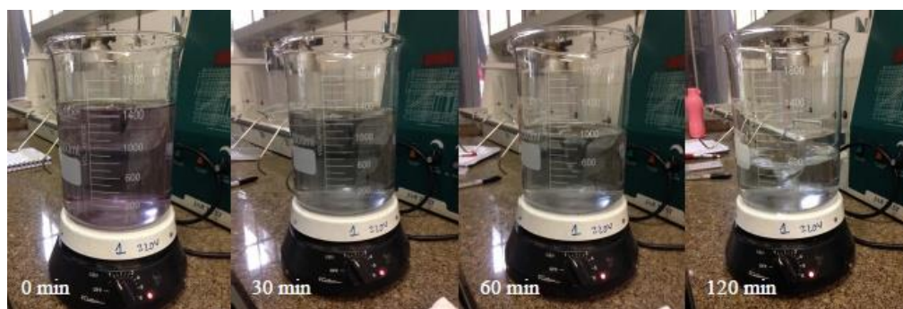
Figure 8: Sample with the application of 40 mg/l of PAC and 1 mg/l of KMnO 4 at times 0, 30, 60 e 120 minutes.
